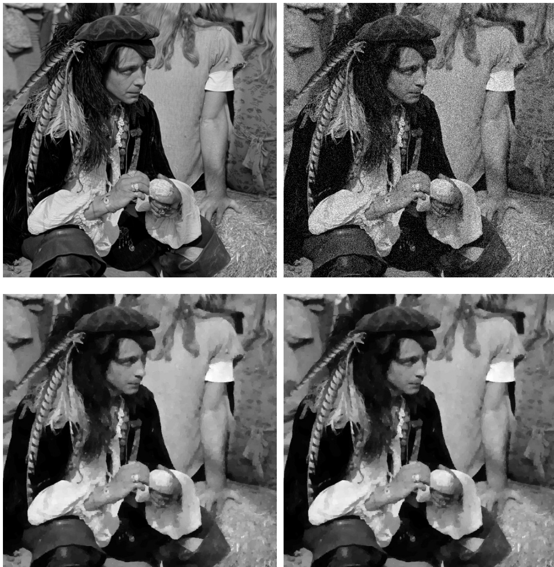
Figure 3.1: Denoising of Man. (top left) Original image. (top right) Noise contaminated with variance 0.01. (bottom left) Denoised with Projective, the stopping criterion was satisfied at iteration 14 (2.313). (bottom right) Denoised with SB, the stopping criterion was satisfied at iteration 16 (2.540).
