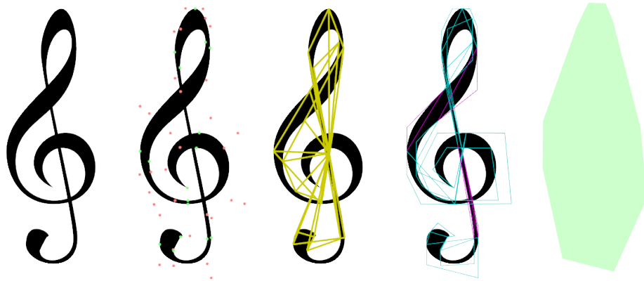
Figure 2.5: The geometry yield by the baking process. From left to right: the path to be filled, its control points, the triangle fan, the discard geometry for curved segments, the conservative covering geometry.
