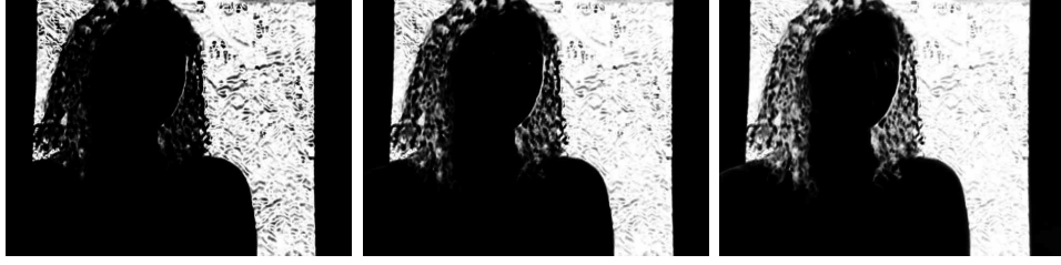
Figure 5.4: Images of background probabilities. Darker pixels have smaller probabilities (left) \sigma_L = 15 (center) \sigma_L = 25 (right) \sigma_L = 35 .
