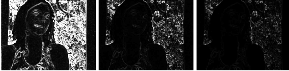
Figure 5.6: Image of boundary probabilities taking the maximum value of a 8-connected neighborhood. Darker pixels have smaller probabilities (left) \sigma_C = 5 (center) \sigma_C = 15 (right) \sigma_C = 25 .
