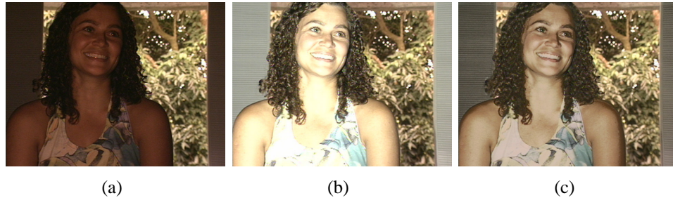
Figure 1.3: Images (a) and (b) are two subsequent video input fields. In this experiment a video camera synchronized with a digital projector acquire images with modulated projected light intensity. In (c) it is shown the tonal-enhanced foreground produced from processing together both (a) and (b) frames.
