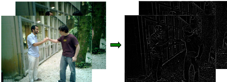
Figure 5.4: Input images shown on the left side, the (amplified x5) result of a High-Pass Laplacian Filter on the right.
