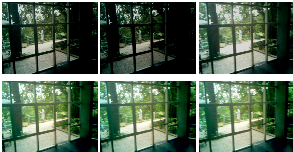
Figure 3.1: (Top) Captured frames. From left to right: optimally-, sub- and super-exposed shots. (Bottom) Corresponding results with tone-mapping.
