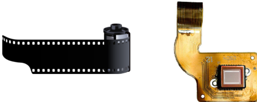
Figure 1.1: In the image above, on the left - chemical photographic film is shown. On the right is a more modern electronic sensor, as present in digital cameras.
