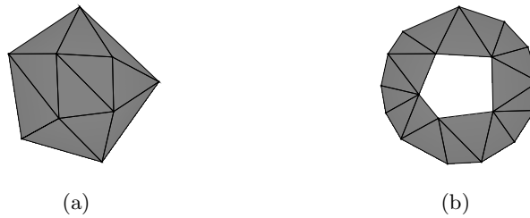
Fig. 1.3: Topology change in the decimation of the ring example. (a) Coarser ring. (b) Finer ring.
