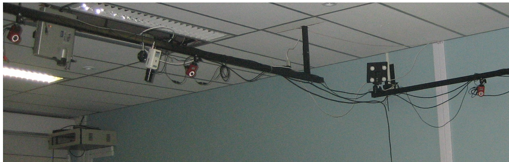
Fig. A.3: OPTITRACK cameras set up at the Visgraf Laboratory.
