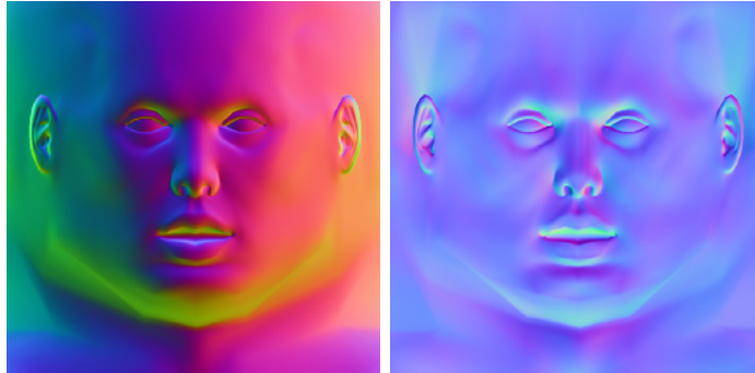
Figure 1.2: Object-space normal maps (left) have range in the unit sphere. Tangent-space maps (right) take values on a single hemisphere. Images taken from [2].
