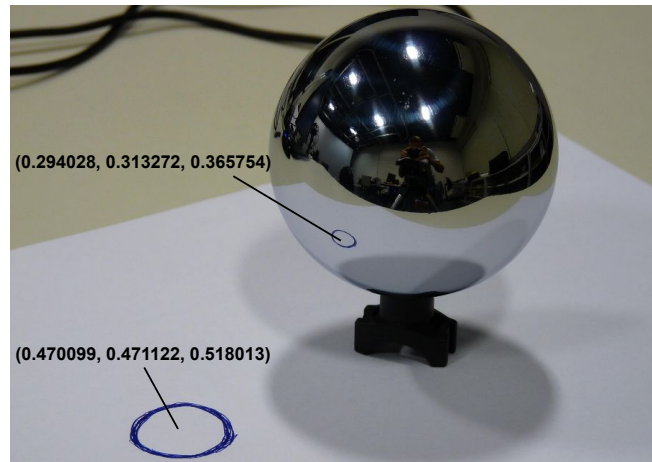
Figure 6.7: The average colors of a white patch in real world and its reflection on the mirrored ball. Dividing these two values you get the reflectivity coefficient of the mirrored ball.
