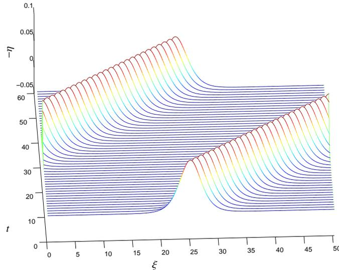
Figure 6: Propagation of a single solitary wave until  $t = 50.8545$ .
