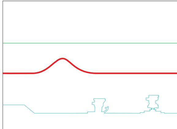
Figure 2: Two-fluid system configuration. Horizontal rigid lid (green), interface (red), bottom topography (cyan).
