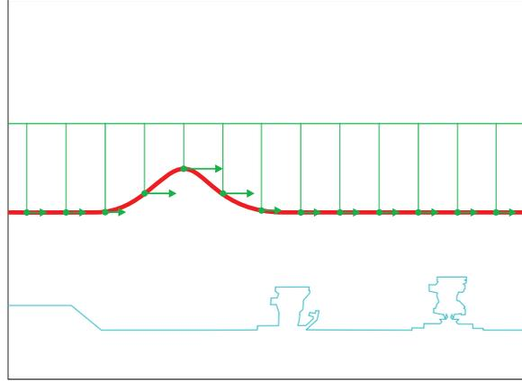
Figure 3: Vertical averaging of physical quantities involved in the upper layer equations. The green arrows indicate the mean-layer horizontal upper velocity  $\bar{u}_1$ .
