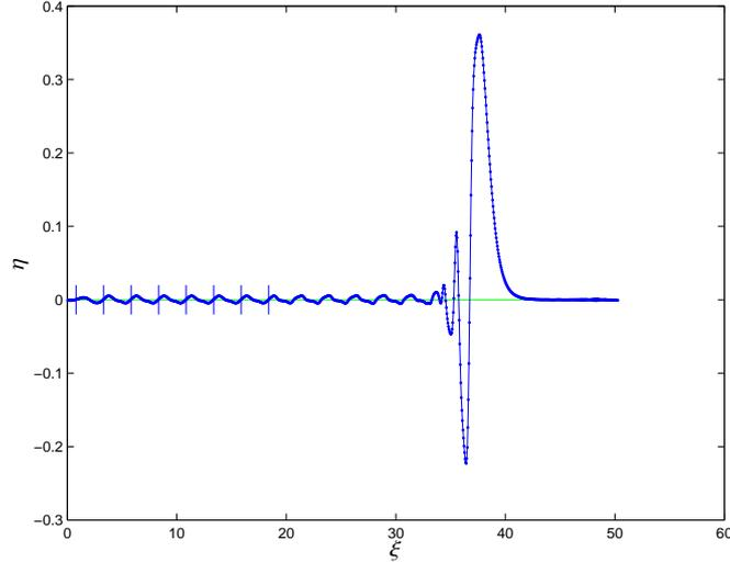
Figure 5: Pulse propagating over a synthetic periodic slowly-varying topography. Dotted line: numerical solution for  $t = 32.3977$ , vertical bars mark spatial intervals of size 2.5133 that fall together with the end of each period of the reflected signal.
