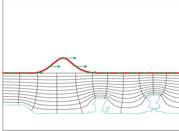
Figure 4: Conformal mapping of the undisturbed bottom layer.
