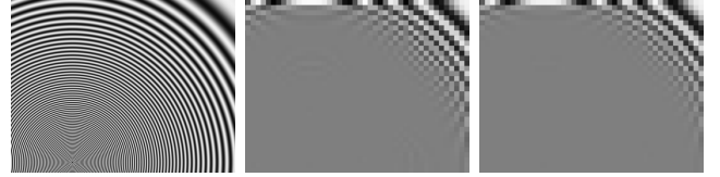
Figure 9: Comparison of aliasing characteristics of two fast downscaling strategies. Given the input image (left), downscaling by a factor of 8 with the traditional Keys filter (70) results in more aliasing (middle) than with generalized downscaling (71) (right).
