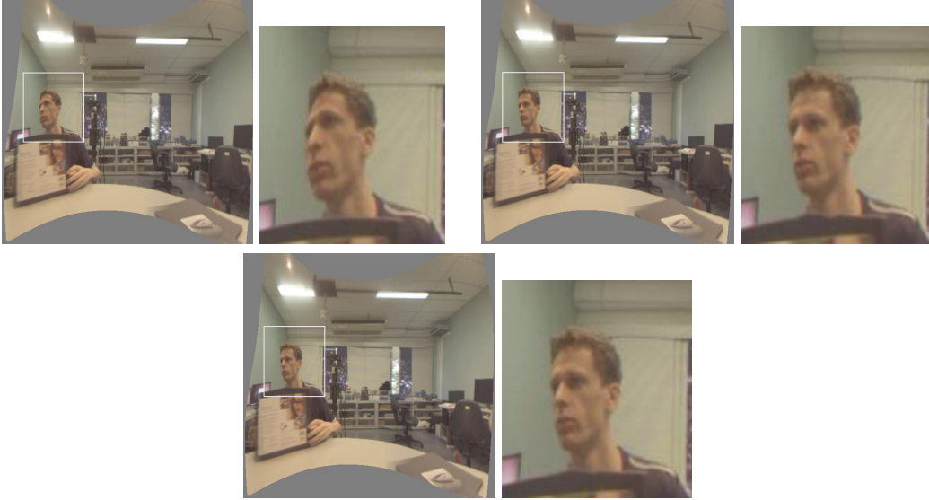
Figure 2: Detail of one frame of the result video after each of the three steps of our method. Top-left: Result video of step 1. The man’s face present unacceptable distortions. Top-right: Result video of step 2. The face is much less distorted, but now some lines near the man are bent. Bottom: Result video of step 3. The head’s shape is preserved, and the lines are a little more correct.
