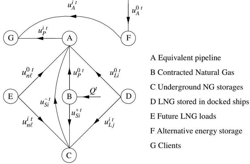
FIGURE 2. Variables controlling the multi-commodity flow in the network
